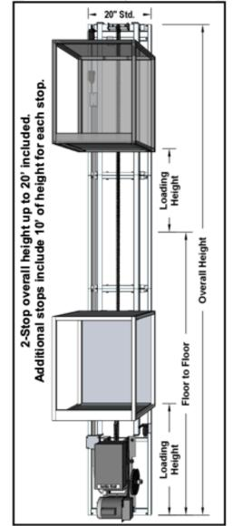
3/4 HP, 110 V, 60Hz motor UL classified elevator controller Powder coated car, rail assembly, and trolley Call / Send stations Door locks & door safety switches (Hoistway doors are not included) Safety switch for motor access panel/door
