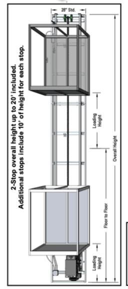
1 HP, (208 V, 230 V, or 460 V), 60Hz, 3 phase motor UL classified elevator controller ASME A17.1 compliant Powder coated car, rail assembly, and trolley Call / Send stations 1 emergency stop button Elevator interlocks (Hoistway doors are not included) Safety switch for motor access panel/door Adjustable limits Top and bottom final limits
